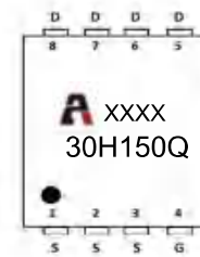
Marking and pin Assignment
